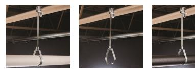
The 115 Standard Duty Loop Hanger is ideal for suspending stationary, non-insulated pipe lines, including CPVC pipes, in fire sprinkler systems. A knurled insert nut helps simplify vertical adjustments and flared edges on the base (1/2" to 4" sizes) help protect pipes from coming into contact with any sharp edges of the hanger.
