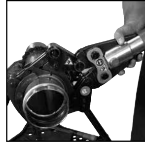
Figure 8: Placement of adapter jaw into pressing chain
