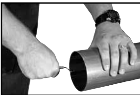
Figure 3: Deburr inside diameter deburring tool
