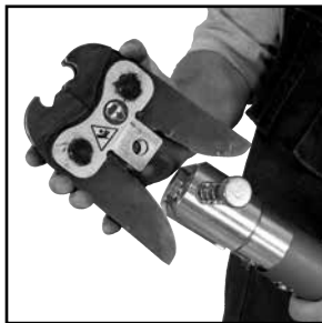
Figure 7: Placement of adapter jaw into the tool
