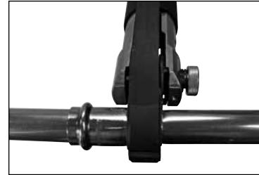
Figure 8 — Jaw set should be square to tubing
