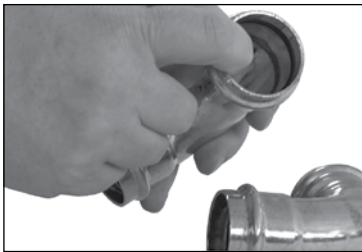
Figure 2 — Check for EPDM Seal
