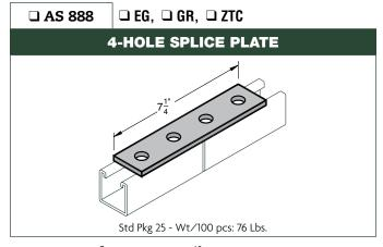
Page notes unless otherwise specified:  $\frac{1}{4}$ " thick,  $\frac{15}{8}$ " wide, holes  $\frac{9}{16}$ " diameter, spaced  $\frac{17}{8}$ " on center and  $\frac{13}{16}$ " from end.
