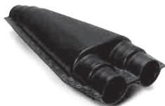
**Protective Y Casing for R-flex** - For waterproof sealing and insulating of dual to single connections. Includes 2 HDPE halves, insulation, sealer kit, and bolts. Must add shrink caps to seal ends of R-flex
