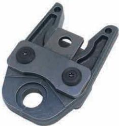
**Power Tool RadiantPEX crimp jaws** are used for crimping PEX tubing and fittings with copper crimp rings. Jaws are available for 3/8" through 1-1/2" sizes of PEX and fittings. These jaws fit our REMS-Akku Press and PowerPress-E power tools, as well as Ridgid 320-E and CT400 power tools. They do not fit the Ridgid 100-B or 210-B power tools.
