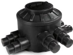
**Protective Inspection Chamber for R-flex** - Allows access to connections and/or valves. Includes HDPE chamber with 6 connection points, inspection lid, sealer kit and screws.
