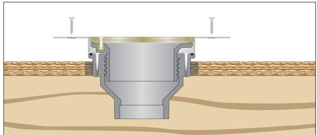
The Halo installs easily from the top side of the floor. Cut a 6" hole and secure with screws or nails.
