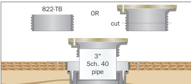
**Using Pipe:** Use the 822-TB or cut the head adapter across the threads. Glue a measured length of 3" Sch. 40 pipe between the two parts with solvent cement.
