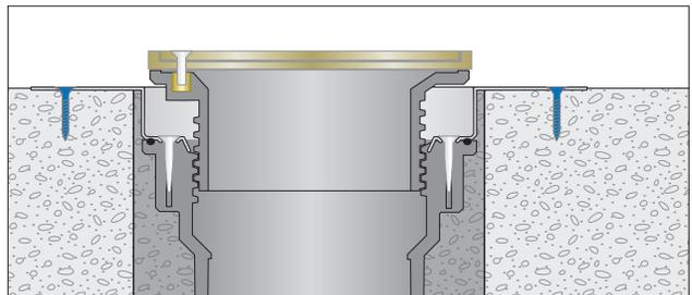
The Halo installs in a 6" cored (single) hole.
