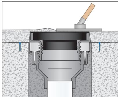
Finish secondary slab flush with the top surface of plug/sleeve assembly.
