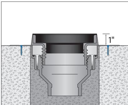
The FinishLine option allows adjustment after the pour. Set the Halo in place and the FinishLine plug/sleeve assembly sets 1" above the deck.
