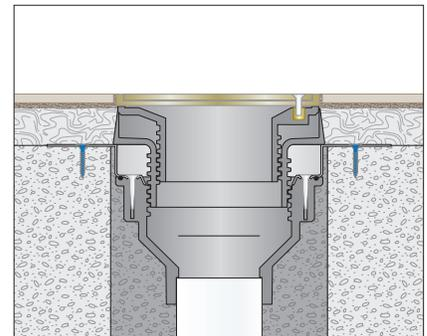
Remove the Coring Plug and replace with the Finish Fixture. The Finish Fixture can be adjusted up to another 1" after the secondary pour.
