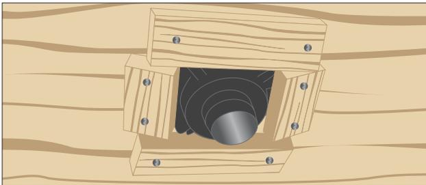
Blocking up a standard drain (with wood or strut) from under the floor is difficult and time consuming.
