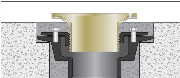
Standard drains require a more costly double-core in concrete slabs.
