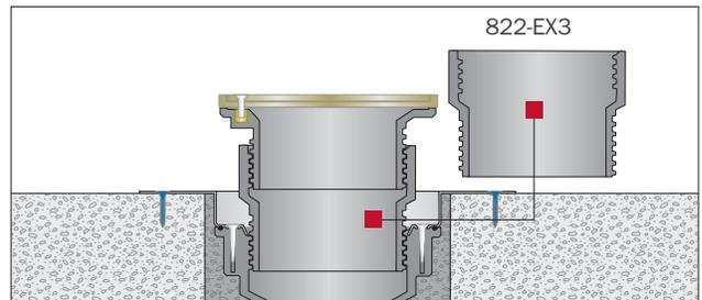
**Extension Adapter:** The 822-EX3 extension adapter installs between the Halo base and the head adapter. Stack multiple adapters if needed.
