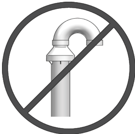
Figure 5-5 Do Not Install U-Bend to Rain Cap
