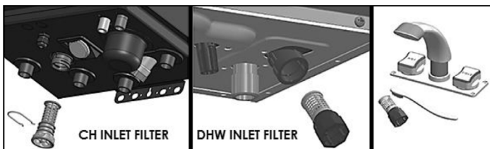
Figure 58 - Cleaning the Inlet Filters
