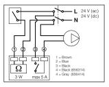
The auxiliary micro-switch shuts off at an average actuator opening value of 80%.
