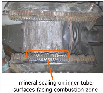
The estimated increase in fuel use due to scale formation, based on research at the University of Illinois and U.S. Bureau of Standards, is shown in figure 2-6.
