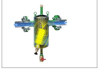
For the steel DIRTMAG<sup>®</sup>, the ferrous impurities are captured by a concentrated magnetic field created by a stack of neodymium rare-earth magnets positioned inside a brass dry-well below the flow stream.
