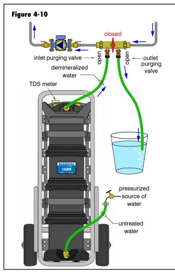
Untreated water from a pressurized source passes through a short hose connected to the bottom hose connection on the HYDROFILL. It is demineralized as it flows upward through the resin beads and exits from the upper hose connection. It flows through another short hose to the inlet purging valve on the system.
