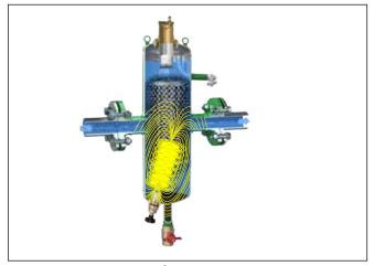
For the steel DISCALDIRTMAG<sup>®</sup>, the ferrous impurities are captured by a concentrated magnetic field created by a stack of neodymium rare-earth magnets positioned inside a brass dry-well below the flow stream.
