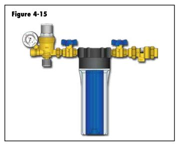
This assembly uses a special 10-inch cartridge insert containing the color changing resin beads necessary to demineralize water passing through it at relatively low flow rates. The cartridge assembly can be isolated by closing the two ball valves. The clear housing can then be unscrewed to remove and replace the cartridge.
