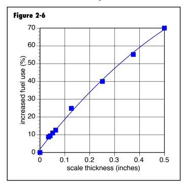
heat exchanger. Any of these can ruin the boiler's heat exchanger and lead to a costly replacement.
