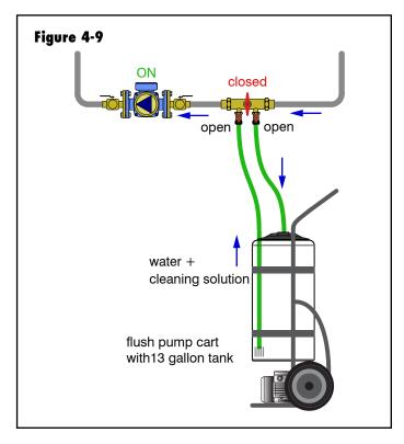
Turn on the flush pump and open both the inlet and outlet purging valves. The inline ball valve should remain closed. The cleaning solution will be injected into the system as an equal amount of water comes back into the tank.
