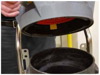
The body is designed to hold highly permeable bags containing the resin beads needed to demineralize water. These bags are simply lowered into the top of the body, as shown in figure 3-4.
