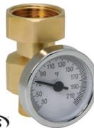
Point of distribution mixed temperature gauge adaptor fits MixCal™ 521 series mixing valves. Threaded union mounting replaces existing mixed outlet with ¾" or 1" sweat pipe connection.
