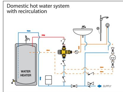
\*MixCal series 521 thermostatic mixing valves with inlet check valves, "AC" models, can be used instead of separately installed check valves.
