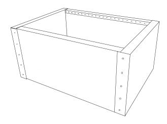
The AirScape Acoustic Plenum will help reduce the over-all sound levels of your Whole House Fan by up to 3 dBA depending on model, fan speed, and installation. We achieve this sound reduction by lining the plenum box with 1.5" thick sound absorbing duct board and by moving the whole house fan farther away from the living space.
