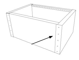
**STEP 6:** Lay a bead of caulking on the top of the framed opening and position the plenum box over the rough opening in the attic. Turn the 4 mounting tabs down into position and secure with the provided wood screws.
