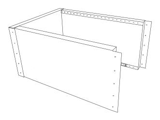
**STEP 4:** Install the remaining end piece and fasten with 5 sheet metal screws on each side.
