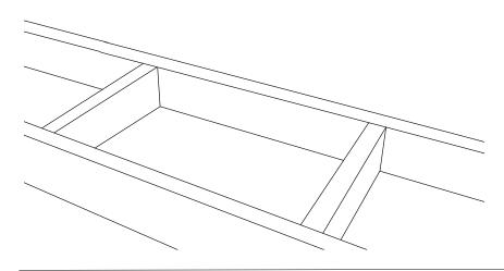
**STEP 2:** Inset 1 of the plenum box sides into 1 of the plenum box ends. Fasten together with 5 of the provided sheet metal screws. The mounting tabs on the side piece should be at the bottom and the side piece should slide into the inside of the end piece.
