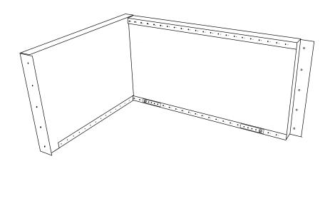
**STEP 3:** Inset the remaining side piece into the end side from step 2. Fasten with 5 sheet metal screws. Note that the mounting tabs should be at the bottom.
