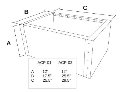
**STEP 1:** Frame out the rough opening for the Whole House Fan per the units installation manual (ACP-01: 14.5" x 22.5" ID) or (ACP-02: 22.5" x 26.5" ID).
